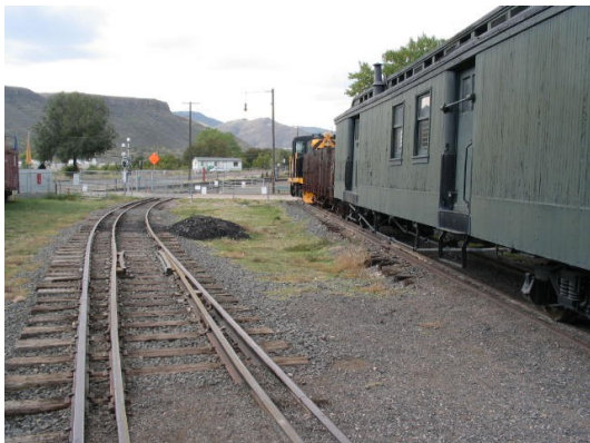
Three rail track. Outer rails are Standard while right two are Narrow Gauge.
